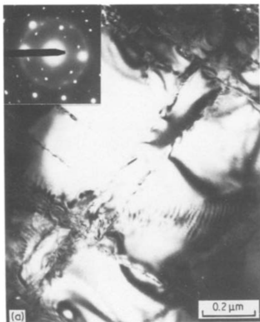
Figure 11 (a, b) Transmission electron micrographs showing recrystallized grains due to extensive plastic deformation and heating of particle interiors.
